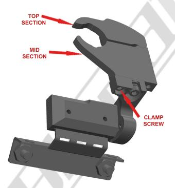
STEP 3 - Loosen the clamp screw so the top section seperates from the mid section. This will provide the necessary clearance to slide the mount over the mirror stem as shown above. Adjust the mirror paralell to the windshield and slightly upward for ease of installation.
