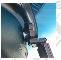
**STEP 6 -** Rotate the mount so it is parallel with the bottom of the mirror. Tighten the clamp screw untill the mount is securely attached to the mirror stem.
