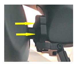
STEP 5 - Position the mount as far forward as you can. Tighten the clamp screw untill the Top and Mid Sections are slightly snug around the mirror stem. You should still be able to rotate the mount.
